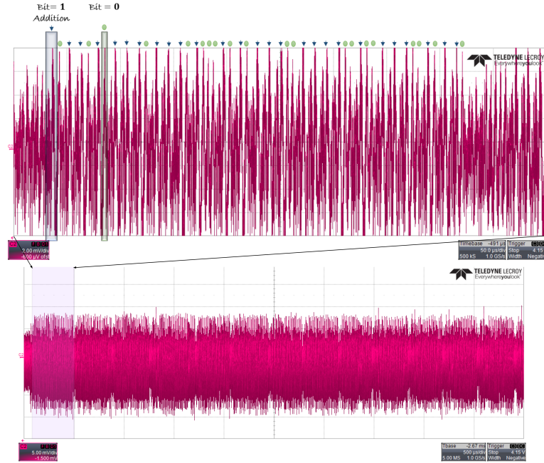
Fig. 4. SPA performed on the first column during Gaussian elimination process
