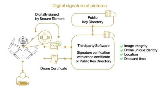
In other words, the digital signature secures all data relevant to a picture, including the place where and the time when it was taken, and by which ANAFI Ai drone.
