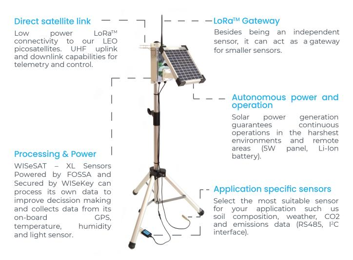
Application: an industrial sensor requires two-way communication to the satellite from remote locations and long endurance without maintenance. This solution can be independent or serve as a gateway for WISeSAT smaller devices that cannot directly reach satellites. Its a gateway for a mass deployment of animals, agricultural sensors, infrastructure monitoring or energy sector.
