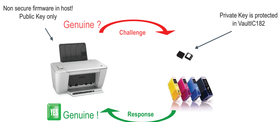
Figure 2 Asymmetric cryptography used in VaultIC182
